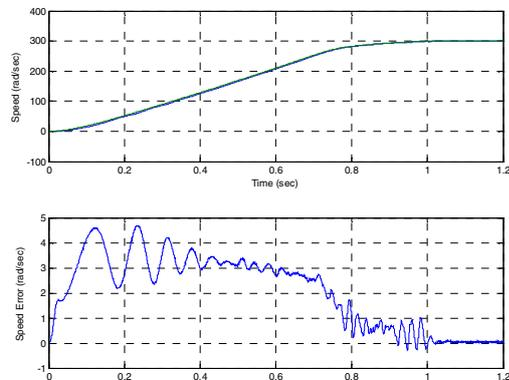
**Fig. 5.** The estimated speed, the motor speed, and the error between the two speed for  $T_r = 0.8*(Tr)n$ .
