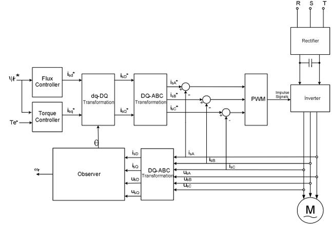
Fig. 3. Block diagram of sensorless speed control.
