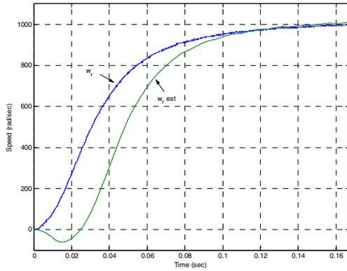
**Fig. 9.** The estimated and the measured speed for 500 rpm of reference speed.
