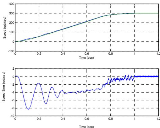
**Fig. 6.** The estimated speed, the motor speed, and the error between the two speed for  $T_r = 1.5*(Tr)n$ .
