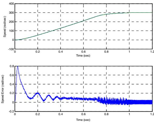
**Fig. 4.** The estimated speed, the motor speed, and the error between the two speed for  $T_r = (Tr)n = 0.0744$ .
