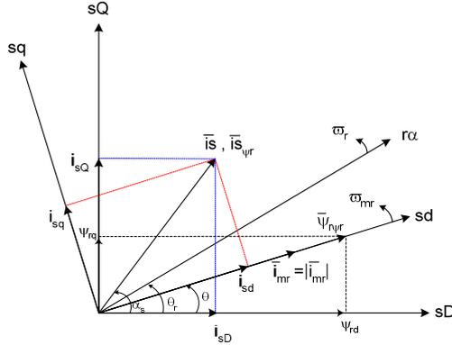
Fig. 1. Stator currents in D-Q and d-q axis.
