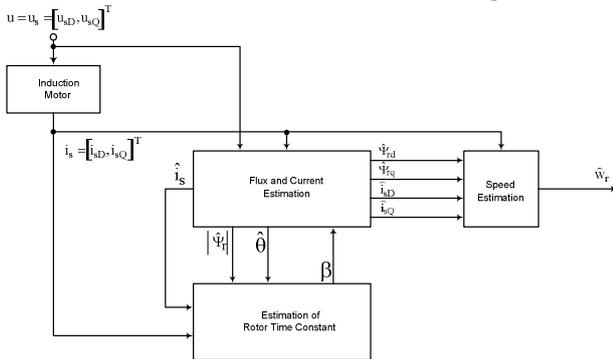
Fig. 2. Block diagram of the speed estimation.
