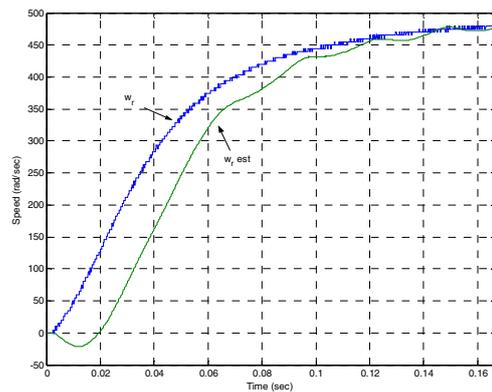
**Fig. 8.** The estimated and the measured speed for 250 rpm of reference speed.
