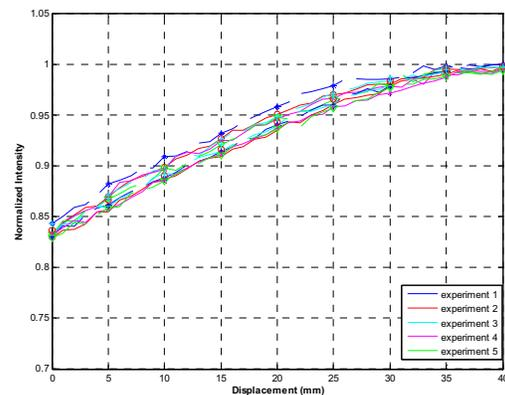
**Fig. 7.** Repeatability test results of the macrobending fiber optic sensor constructed using 7 loops of 62.5/125  $\mu\text{m}$  multi-mode fiber.
