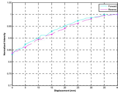
**Fig. 6.** Forward and reverse loading effects of the macrobending fiber optic sensor constructed using 7 loops of 62.5/125  $\mu\text{m}$  multi-mode fiber.
