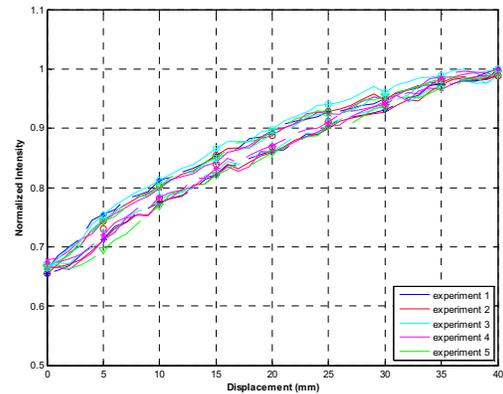
**Fig. 10.** Repeatability test results of the macrobending 62.5-50-62.5 hetero-core fiber optic sensor constructed using 7 loops.
