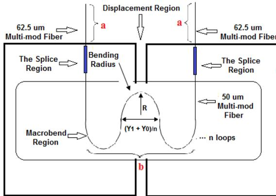
**Fig. 5.** Periodic macrobending sensor configuration with displacement.
