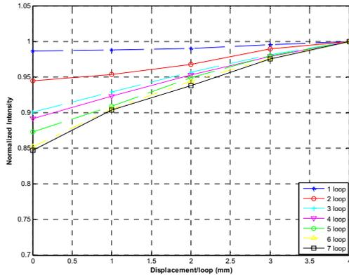
**Fig. 8.** Comparison of forward loading effects for the macrobending fiber optic sensor constructed using different numbers of loops of 62.5/125  $\mu\text{m}$  multi-mode fiber.
