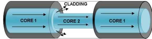
**Fig. 2.** Hetero-core optical fiber structure.
