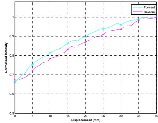
**Fig. 9.** Forward and reverse loading effects of the macrobending 62.5-50-62.5 hetero-core fiber optic sensor constructed using 7 loops.
