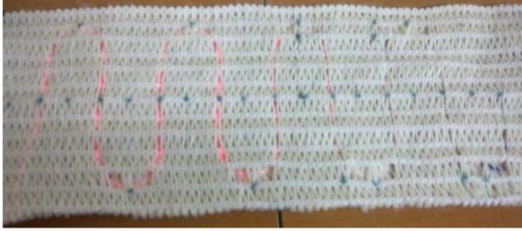
**Fig. 4.** Sensing region of the periodic macrobending fiber optic sensor.
