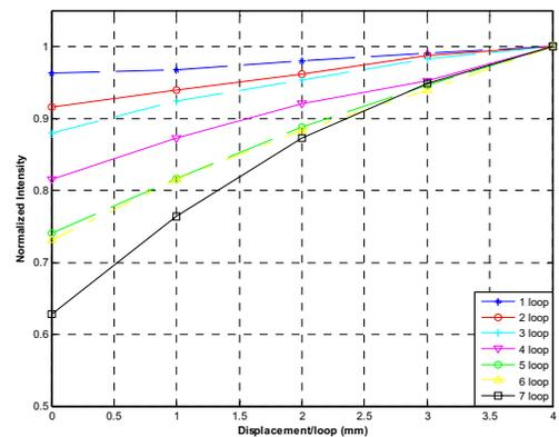
**Fig. 11.** Comparison of forward loading effects for the macrobending 62.5-50-62.5 hetero-core fiber optic sensor constructed using 7 loops.
