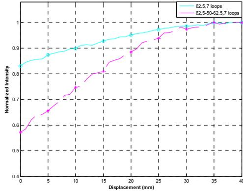
**Fig. 12.** Comparison of forward loading effects for the macrobending 62.5-50-62.5 hetero-core fiber optic sensor and 62.5/125  $\mu\text{m}$  multi-mode fiber optic sensor constructed using 7 loops.
