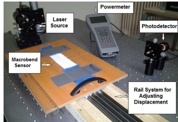
**Fig. 3.** Experimental setup of macrobend sensor.
