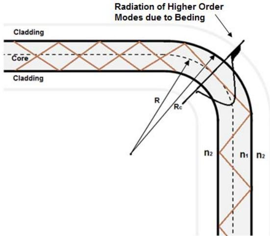
**Fig. 1.** Radiation of higher order modes in an optical fiber due to bending.
