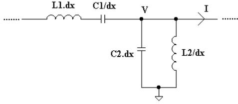
Figure.2 A distributed bandpass transmission line section
