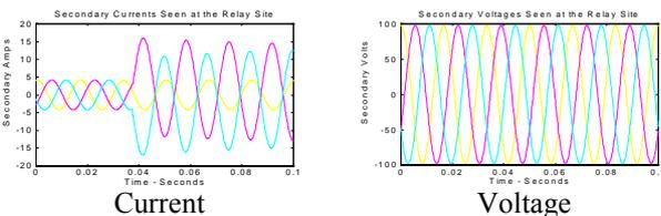
Figure 7: Transient Fault at maximum B-C Voltage
