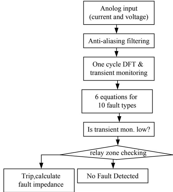
Figure 2: Relay Algorithm Implemented in MATLAB
