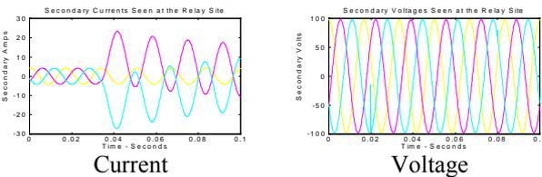
Figure 6: Transient Fault at minimum B-C Voltage
