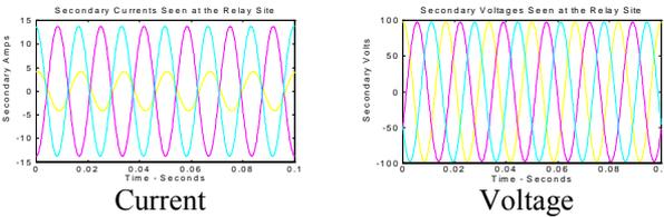
Figure 5: Steady State Forward Fault (Inside of Zone)
