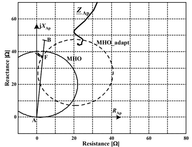
Figure 7. Conventional (solid) and adaptive (dotted) distance relay characteristics and measured impedance trajectory
