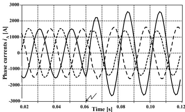
Figure 4. Phase currents at the relaying point – faulted line
