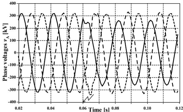
Figure 3. Phase voltages at the relaying point – faulted line
