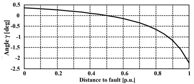
Figure 2. Plot of  $\gamma$  angle variation as a function of a distance to fault
