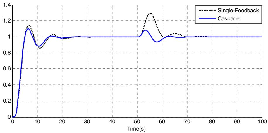
**Figure 3.13:** Unit Step Responses of the Single-Feedback and Cascade Control Systems (PI-PI)
