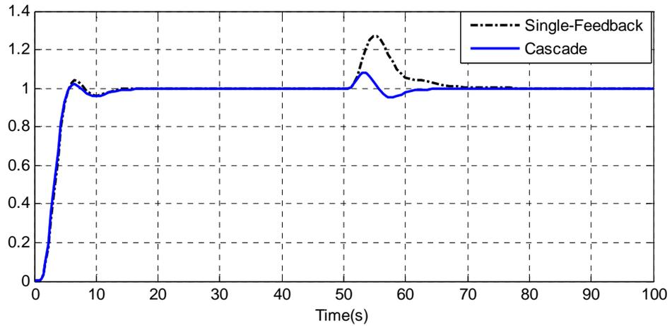
Figure 3.7: Unit Step Responses of the Single-Feedback and Cascade Control Systems (PID-PI)
