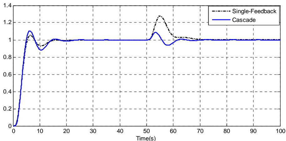
**Figure 4.2:** Unit Step Responses of the Cascade (PI-PI) and Single-Feedback (PID) Control Systems
