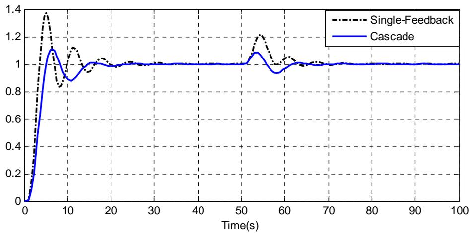
**Figure 3.6:** Unit Step Responses of the Single-Feedback and Cascade Control Systems (PI-PID)
