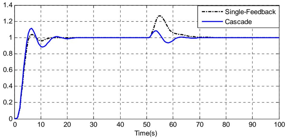
**Figure 3.10:** Unit Step Responses of the Single-Feedback and Cascade Control Systems (PI-PID)
