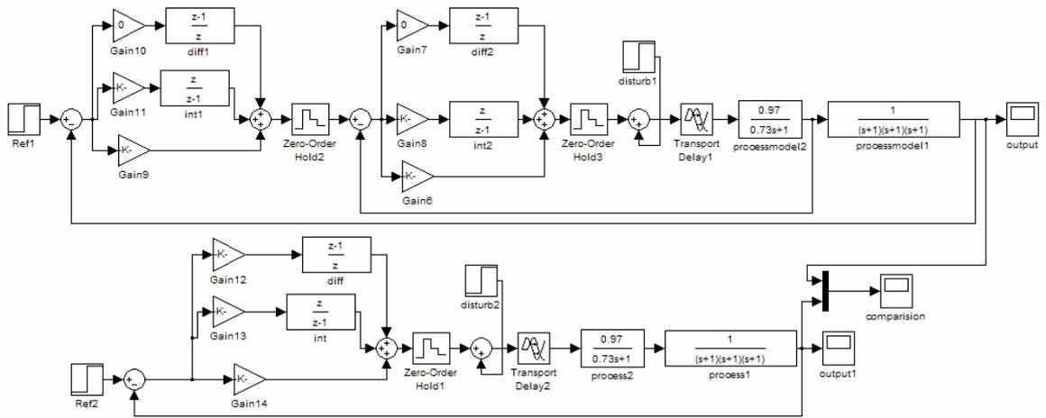
**Figure 4.1:** Simulation Block Diagram for Digital Control
