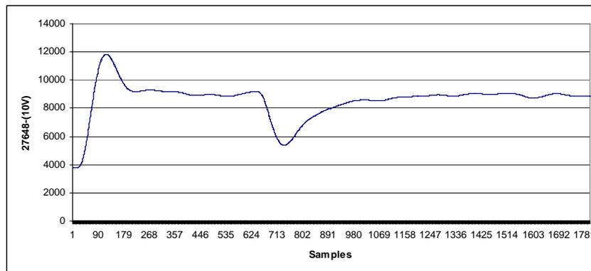
Figure 4.14: Unit Step Response of the Single-Feedback Control System
