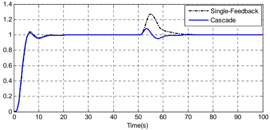
**Figure 3.8:** Unit Step Responses of the Single-Feedback and Cascade Control Systems (PID-PID)
