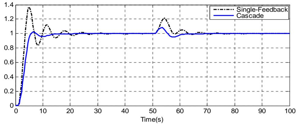
**Figure 3.3:** Unit Step Responses of the Single-Feedback and Cascade Control Systems (PID-PI)
