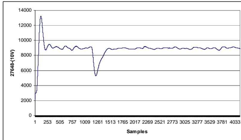
Figure 4.13: Unit Step Response of the Single-Feedback Control System
