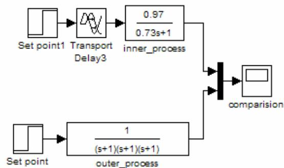
**Figure 4.8:** Simulation Diagram of the Two Systems
