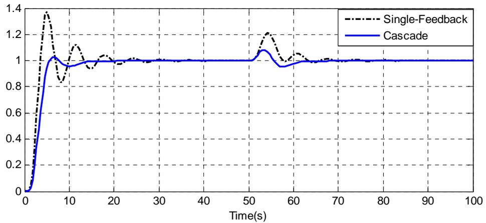
**Figure 3.4:** Unit Step Responses of the Single-Feedback and Cascade Control Systems (PID-PID)
