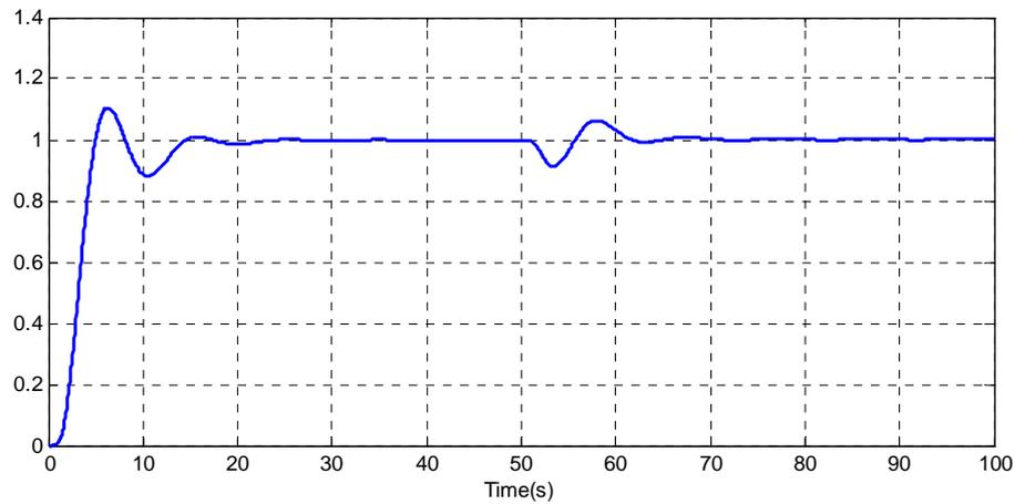
**Figure 4.11:** Unit Step System Response of a Cascade Control System with Negative Disturbance
