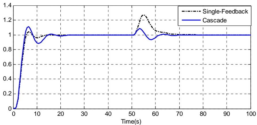
**Figure 3.9:** Unit Step Responses of the Single-Feedback and Cascade Control Systems (PI-PI)
