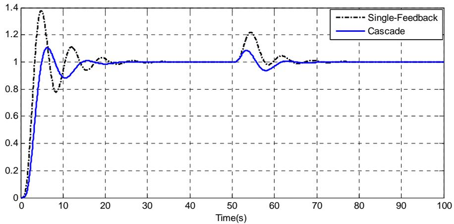
**Figure 4.3:** Unit Step Responses of the Cascade (PI-PI) and Single-Feedback (PID) Control Systems
