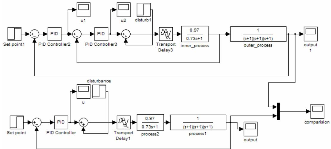
**Figure 3.2:** Simulation Block Diagram of the Single-Feedback and Cascade Control Systems
