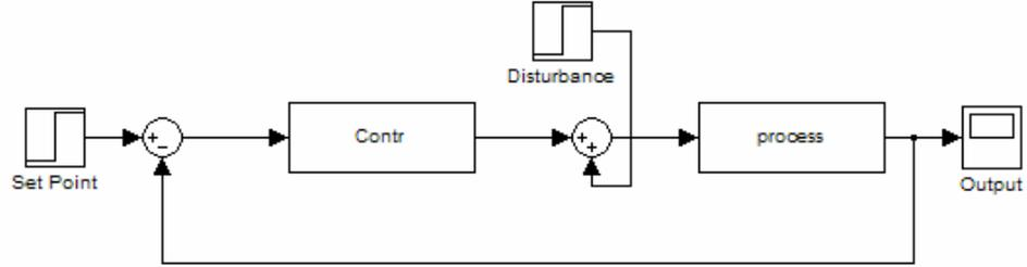
Figure 2.1: Single-Feedback Control System
