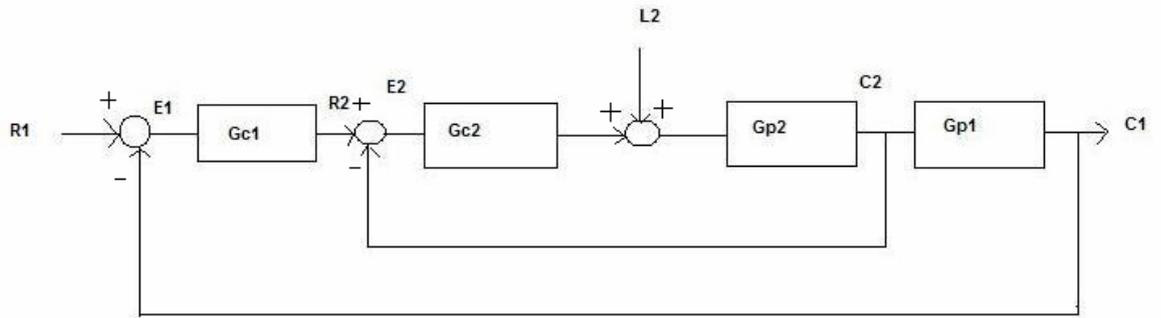
**Figure 3.1:** Block Diagram of the Cascade Control System
