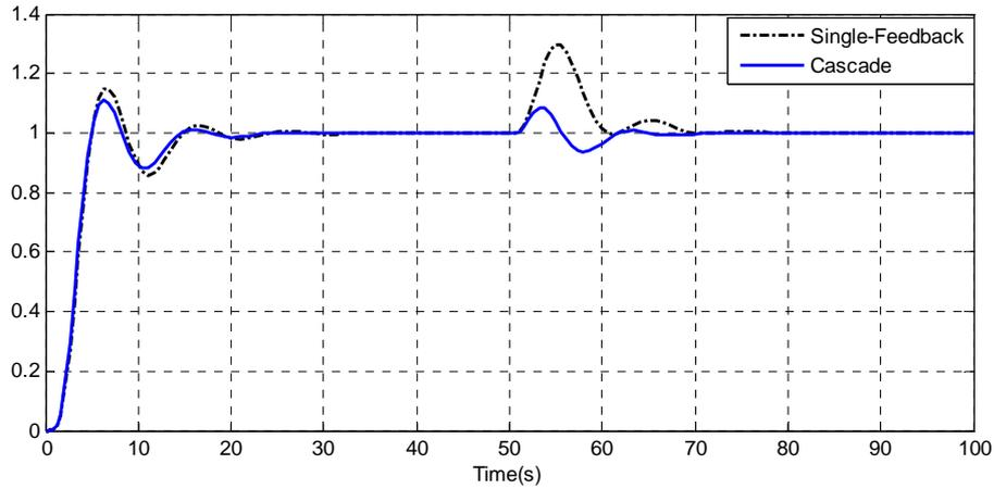
**Figure 3.14:** Unit Step Responses of the Single-Feedback and Cascade Control Systems (PI-PID)
