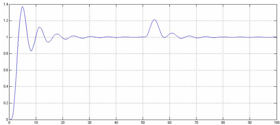
**Figure 2.3:** Unit Step Response of the Controlled System
