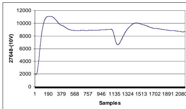
Figure 4.15: Unit Step Response of the Cascade Control System
