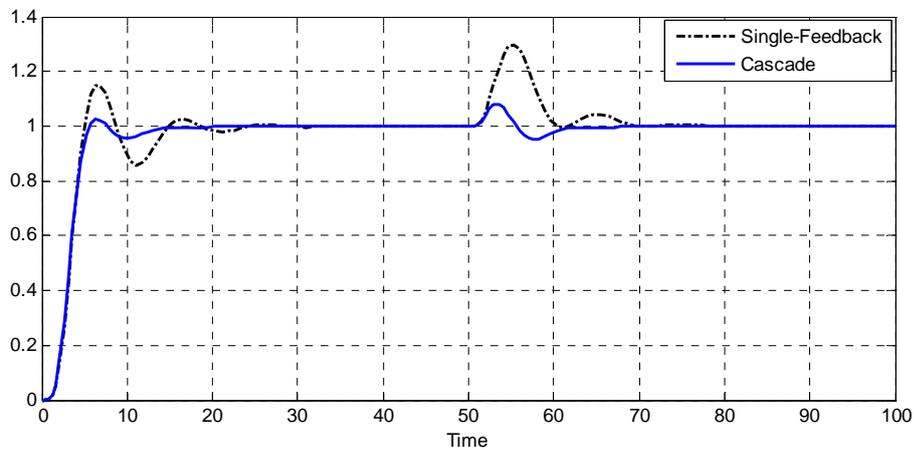
Figure 3.12: Unit Step Responses of the Single-Feedback and Cascade Control Systems (PID-PID)
