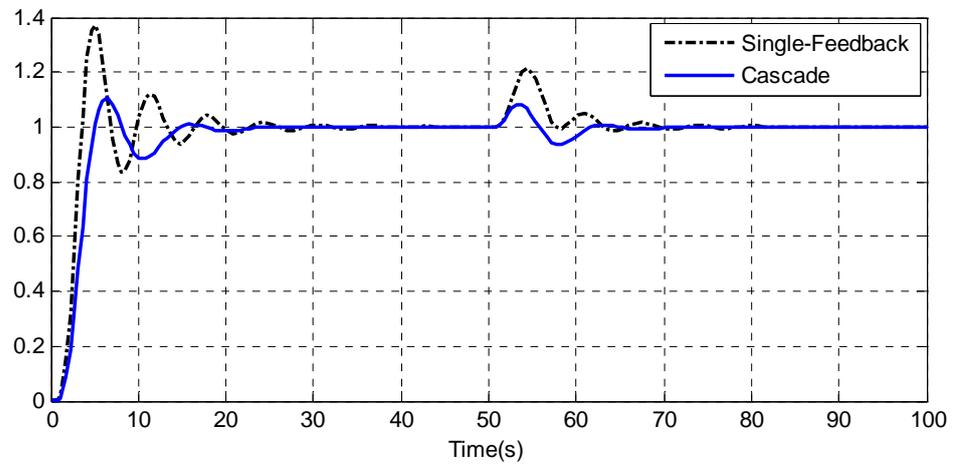
**Figure 3.5:** Unit Step Responses of the Single-Feedback and Cascade Control Systems (PI-PI)
