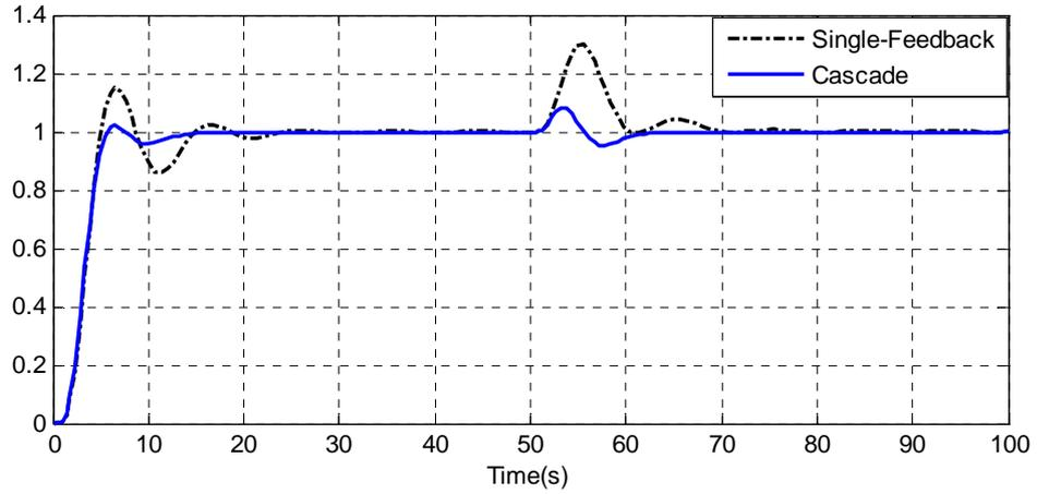
Figure 3.11: Unit Step Responses of the Single-Feedback and Cascade Control Systems (PID-PI)
