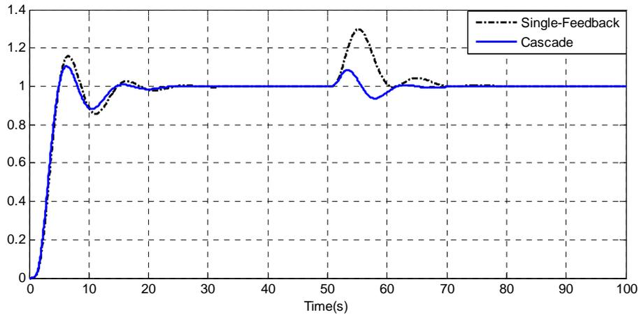
**Figure 4.4:** Unit Step Responses of the Cascade (PI-PI) and Single-Feedback (PI) Control Systems
