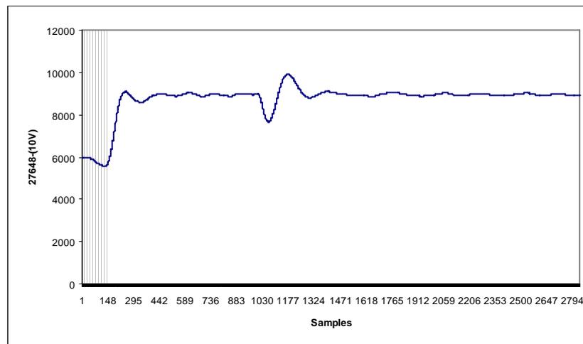
**Figure 4.12:** Unit Step Response of the Cascade Control System
