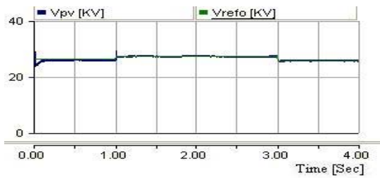
Fig. 9. Photovoltaic panel and reference voltages
