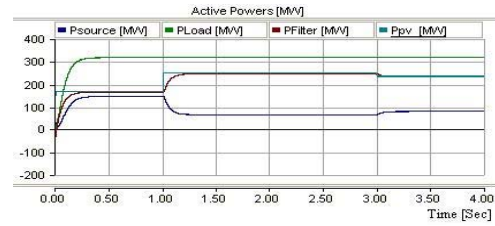
Fig. 12. Active power of load (QLoad) and source (QSource) and Active filter (QFilter), PV (Ppv) sides.
