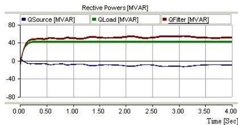
Fig. 11. Reactive power of load (QLoad) and source (QSource), Active filter (QFilter) sides.
