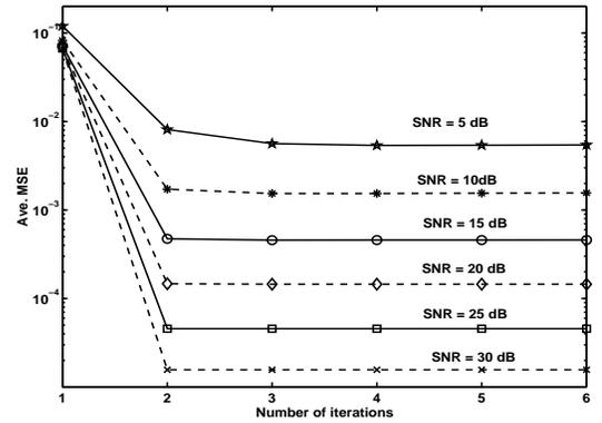
Fig. 4. MSE performance of the EM algorithm as a function of number of iterations ( $\tau_{rms} = 4$  sample for the exponentially decaying power delay profile)
