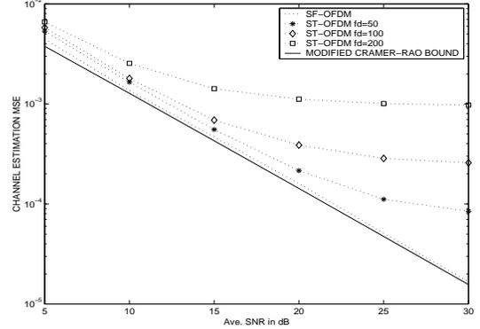
Fig. 3. MSE performance of the EM algorithm as a function of average SNR
