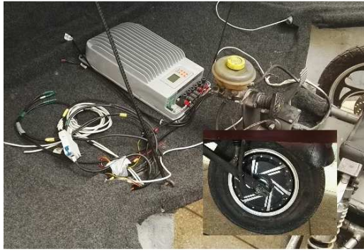
Figure 15 Motor with drive controller
