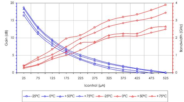
Figure 18 : Gain control of the differential LNA, for different temperatures;  $V_{DC} = \pm 2.5V$   $I_{BIAS} = 1.1mA$
