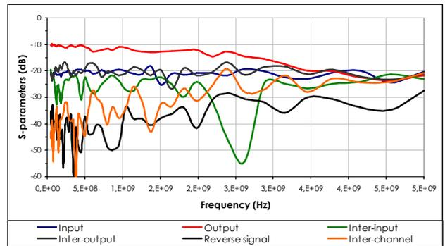
Figure 15 : S-parameters of the differential LNA, for gain = 10dB; at  $V_{DC} = \pm 2.5V$  and  $I_{BIAS} = 1mA$
