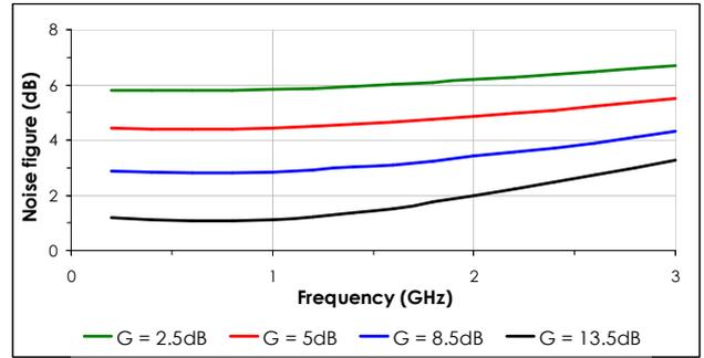
Figure 9 : Noise figure profiles for the single-ended LNA
