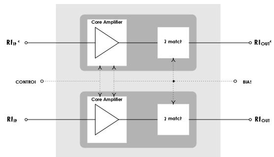
Figure 11 : Block-level description of the new differential LNA
