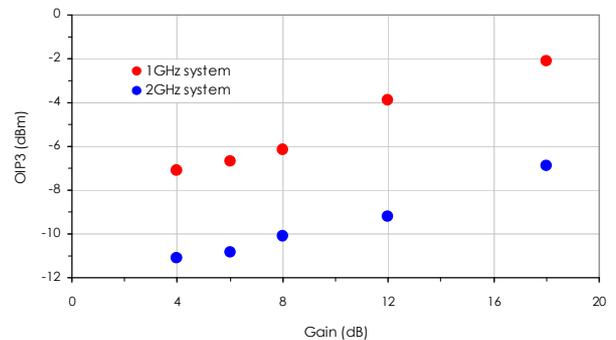
Figure 17 : OIP3 between  $P_1$  and  $P_3$  of the differential LNA as a function of the LNA's gain; at  $V_{DC} = \pm 2.5V$  and  $I_{BIAS} = 1.1mA$
