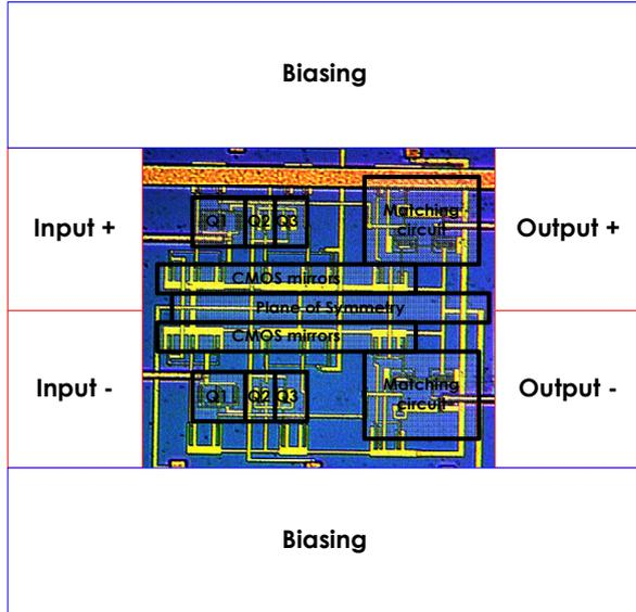
Figure 12: Close-up of the differential LNA showing the signal-chain transistors  $Q_1$  to  $Q_3$ , the output matching circuit and the CMOS mirrors; the two halves are laid out around a symmetry plane
