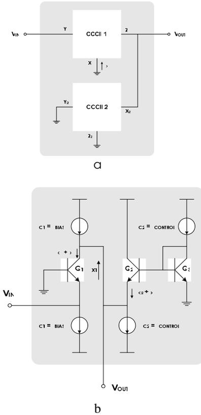
Figure 4 : New CCCII-based Low-Noise amplifiers
