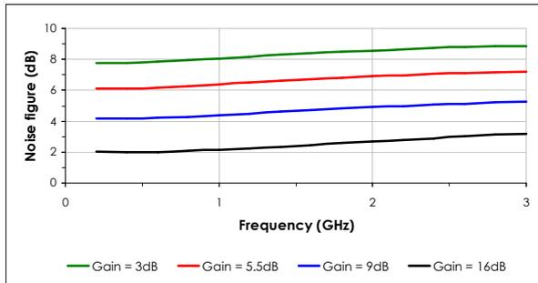
Figure 16 : Noise figure profiles for the differential LNA
