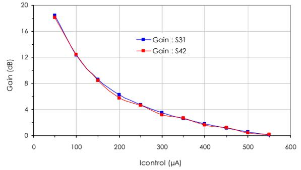
Figure 14 : Symmetry between the two amplification channels of the differential LNA : gain versus  $I_{CONTROL}$ ; at  $V_{DC} = \pm 2.5V$  and  $I_{BIAS} = 1.1mA$
