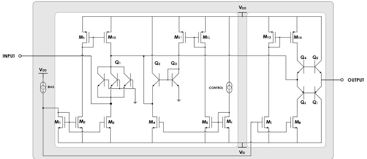
Figure 5 : Complete transistor-level description of a single-ended LNA based on the new principle
