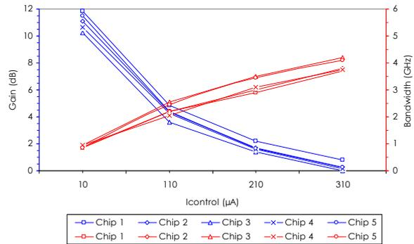
Figure 19 : Gain control and bandwidth of the five LNA prototypes; at  $V_{DC} = \pm 2.5V$  and  $I_{BIAS} = 1.4mA$
