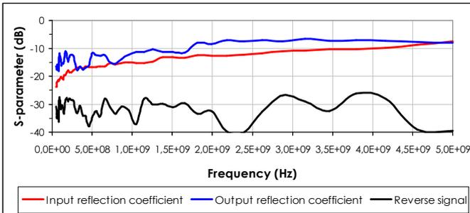
Figure 8 : S-parameters of the single-ended LNA, for gain = 6dB; at  $V_{DC} = \pm 1.5V$  and  $I_{BIAS} = 450\mu A$
