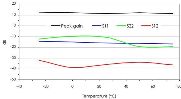
Figure 10 : S-parameters of the single-ended LNA, versus temperature, for gain = 10dB; at  $V_{DC} = \pm 1.5V$  and  $I_{BIAS} = 450\mu A$
