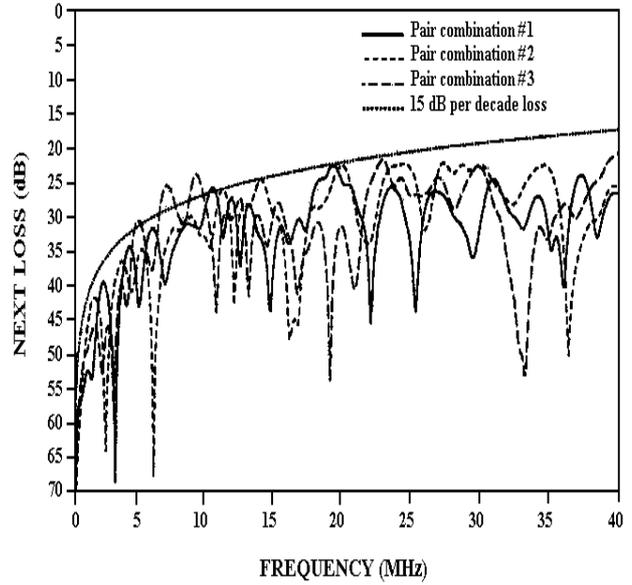
**Fig. 4. NEXT Loss Between Pairs of Category 3 Cables**
