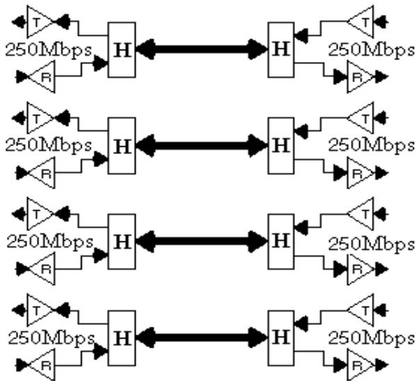
**Fig. 6. Data Transmission in 1000Base-T**
