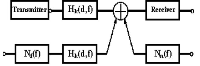
Fig. 2. Channel Model of A Pair
