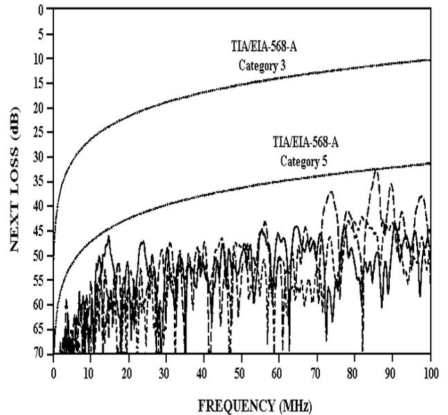
**Fig. 5. NEXT Loss Between Pairs of Category 5 Cables**
