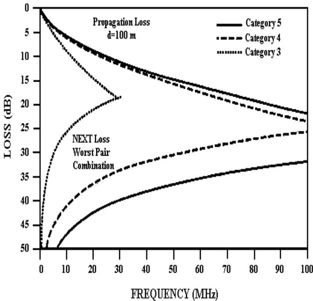
**Fig. 3. TIA/EIA-568-A Worst-Case Propagation Loss and Pair-to-Pair NEXT Loss**
