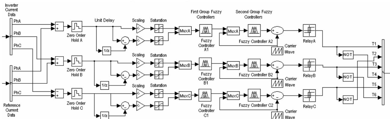
Fig 7. (Hierarchical Current Controller)
