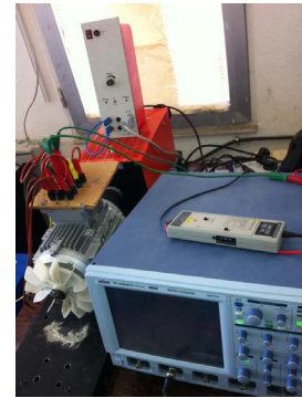
Figure 5. Experimental setup for static air-gap eccentricity based on measuring of voltage between sub-windings of dual three-phase induction motor.
