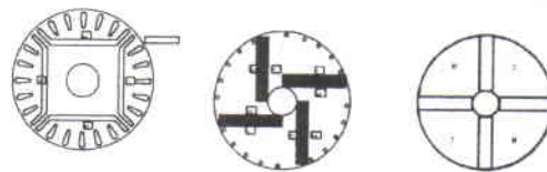
Fig. 1. Examples of salient pole-like rotor designs
